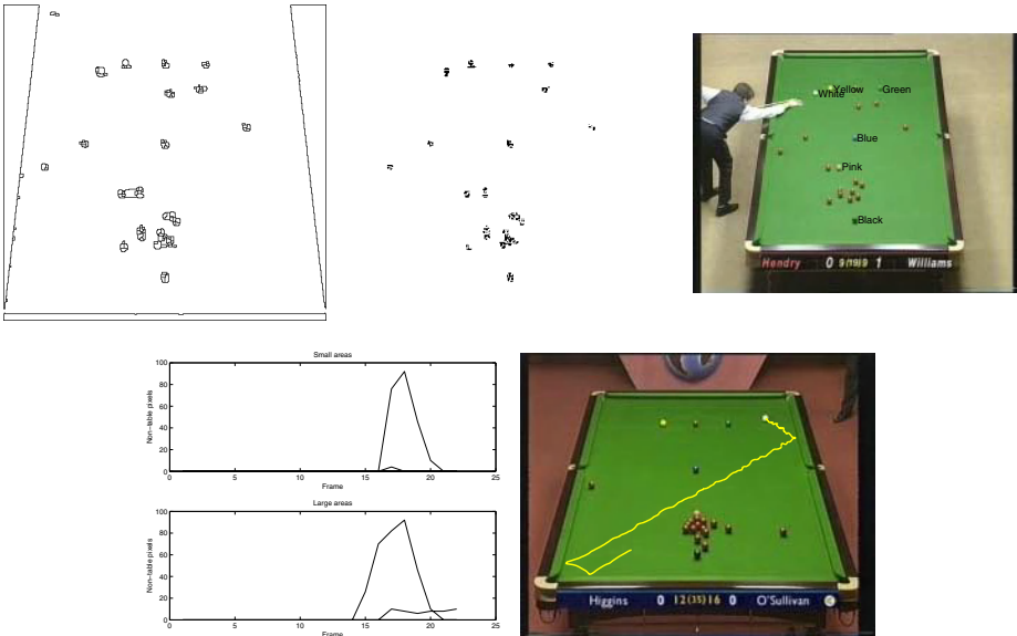
Fig. 3. Top Row: Implementation of the watershed algorithm showing the object map; Superfluous objects removed from the object map; Several balls found and labelled; Bottom Row: (Left) The top figure shows the small region around the pocket and the bottom one is the surrounding region. The ball enters the larger region first and subsequently the smaller one. The peaks decrease simultaneously in both indicating that the ball has been potted. The smaller peak in both traces is due to player occlusion. (Right) Ball tracking via CONDENSATION
