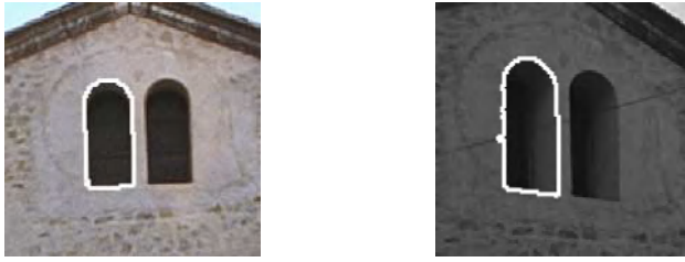
Fig. 3. Covariant regions II. MSE (see main text) regions (outline shown in white) detected in images from the data set illustrated by figure 1. The change of view point and difference in illumination are evident but the same region has been detected in both images independently
