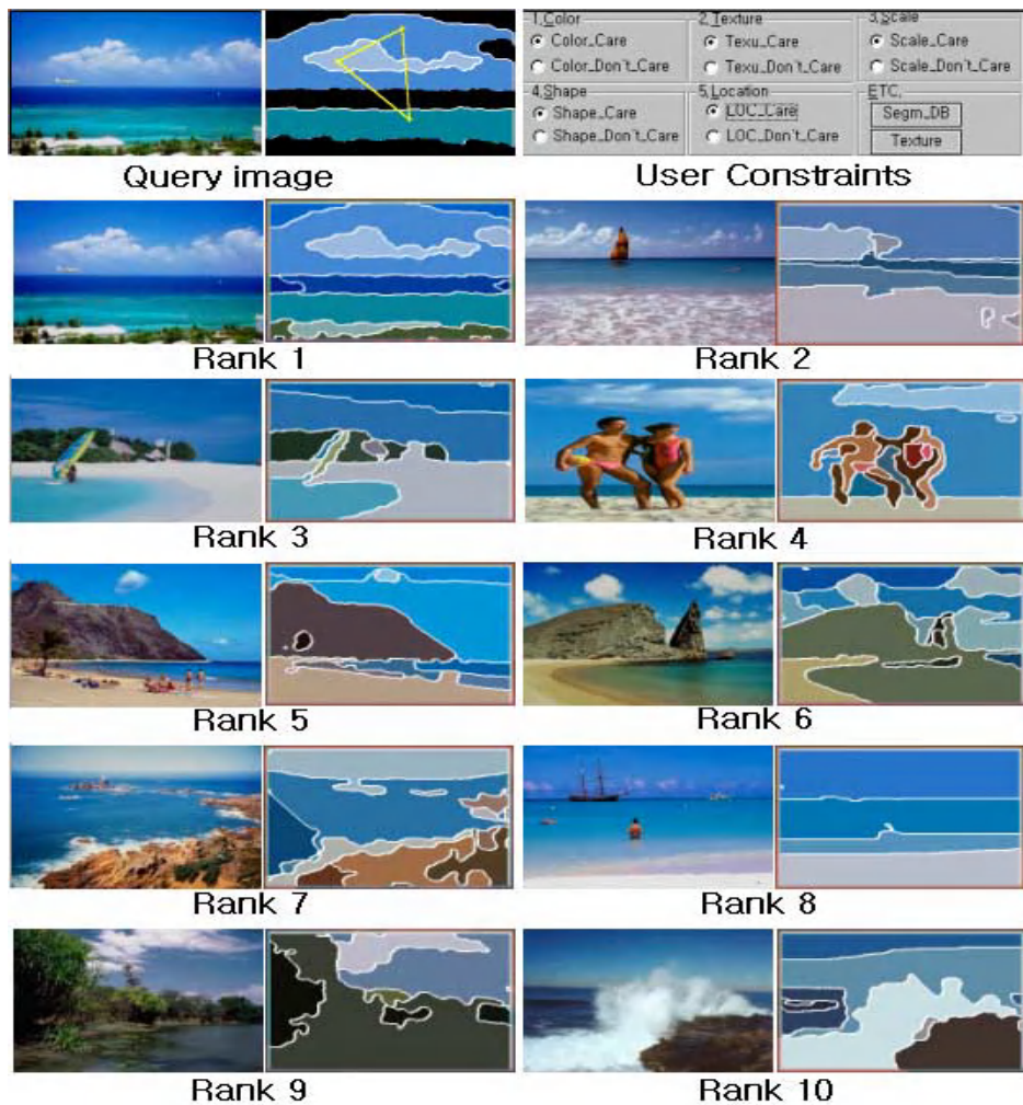
Fig. 6. Retrieval results after five iterations: Query region – blue sky with a white cloud and sea (left: original image, right: query regions and their spatial relationships). As shown in retrieval results, our method permits deletion or insertion of regions
