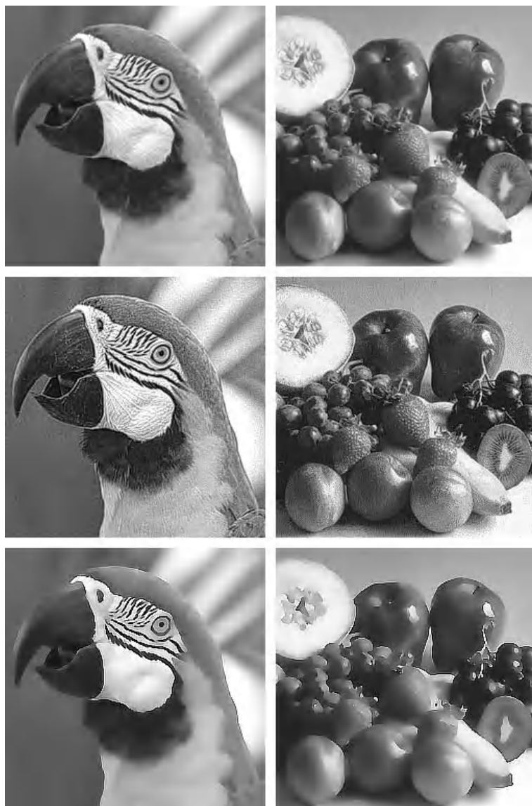
Fig. 5. Illustration of the new combined forward and backward anisotropic diffusion scheme. Top: color test images, below images enhanced with the pure backward diffusion and at the bottom images enhanced with the FAB diffusion scheme presented in the paper
